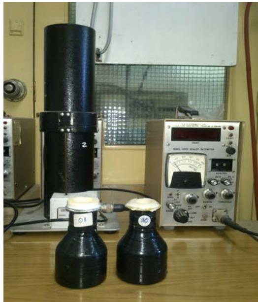
**Figure 2.** Short term electret and ionization chamber configuration (SST), and Scintillation glass vial with activated charcoal
